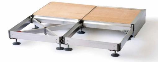
A decorative, flat floor is an element of the equipment of trade fair and exhibition stands. Made of aluminum and wood. In the floor system, it is possible to hide water, electricity and communication cables. The patented folding frame system saves space and is easy to transport. The frames are foldable and equipped with appropriate adjustment feet, and then equipped with wooden platforms.
